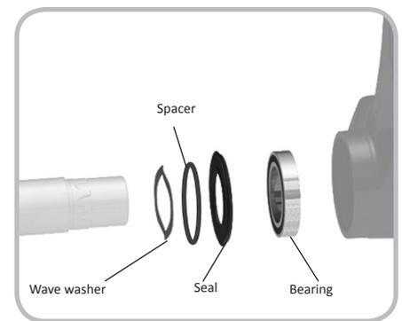
Figure 14.39. SRAM bearing set
