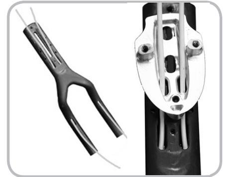
Figure 7.8. Shift housing routed through mono-extension and mono-spacer
