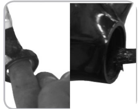
Figure 14.16. Greasing the bearing and the frame seat
