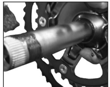
Figure 14.36. Greasing the axle
