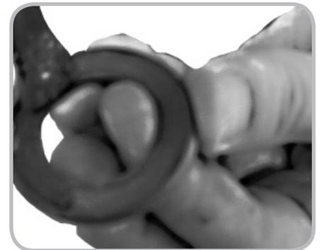
Figure 14.10. Greasing the bearing covers
