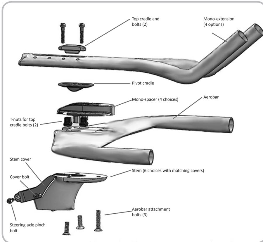
Figure 7.1. Exploded assembly of stem, aerobar, and mono-extension
