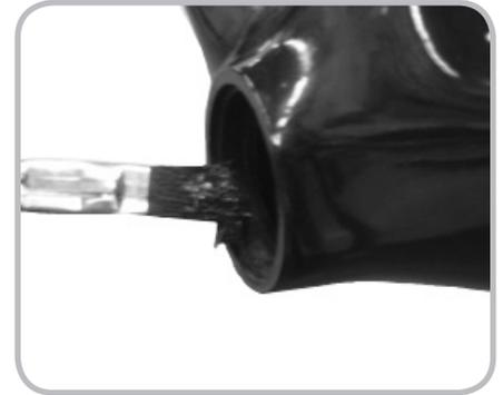
Figure 14.29. Greasing the bearing cups
