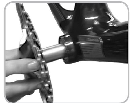
Figure 14.31. Inserting the non-drive side axle
