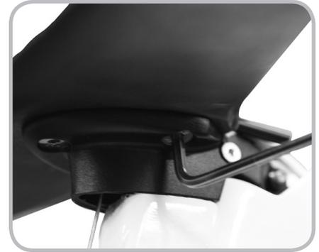
Figure 6.10. Aerobar attachment bolts (three)
