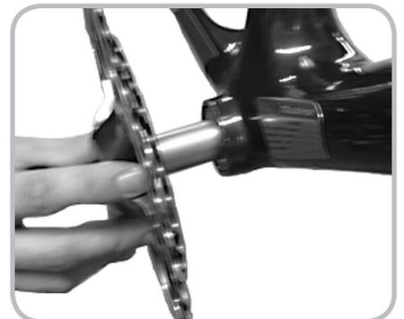
Figure 14.37. Sliding the axle through the bearings
