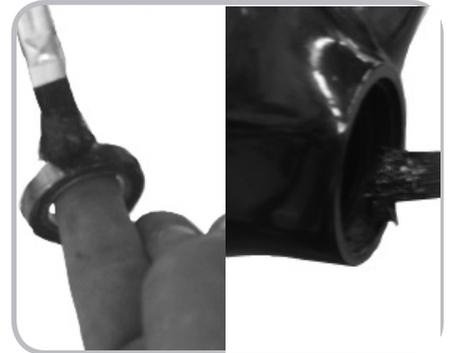
Figure 14.34. Greasing the bearing and the frame saddle
