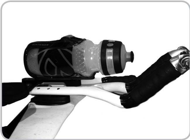
Figure 13.5 Speed Concept bottle cage
