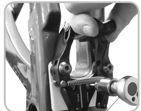
Figure 11.3. Brake attached by two bolts
