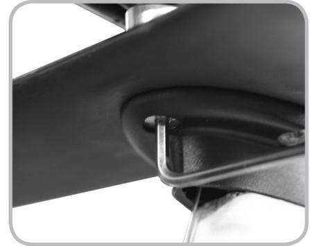
Figure 7.19. Tightening front attachment bolt
