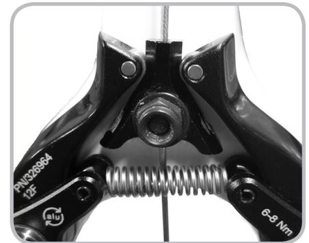
Figure 10.5. Cable in wedge
