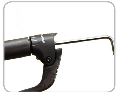
Figure 7.14. Installing brake lever
