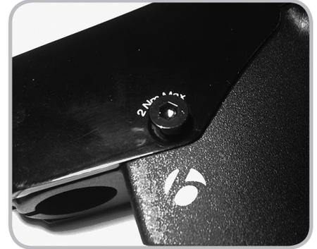
Figure 7.22. Housing cover on stem
