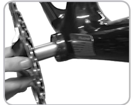
Figure 14.21. Sliding the axle through the bearings
