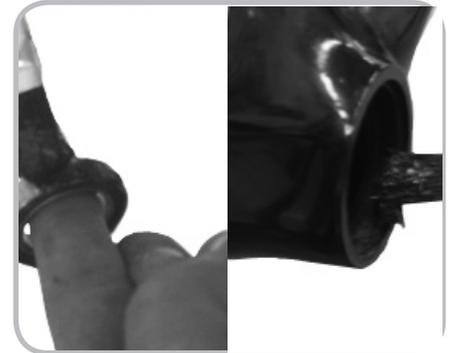
Figure 14.7. Greasing the bearing and the frame saddle
