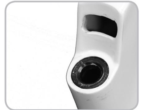
Figure 6.2. Upper head bearing pressed into frame
