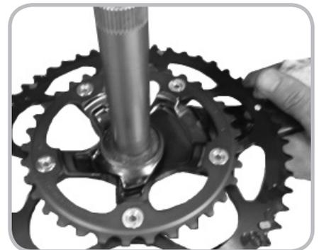
Figure 14.19. Sliding the bearing cover onto the axle
