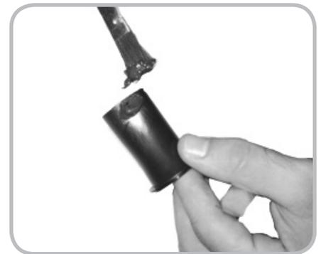
Figure 14.1. Applying grease to the axle shield
