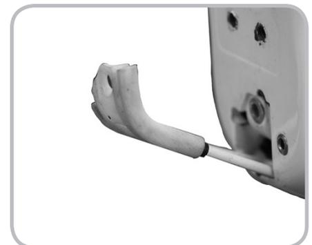
Figure 7.4. Bottom bracket cable guide on shift housing
