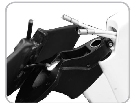
Figure 7.18. Installing the aerobar, ferrule in long position
