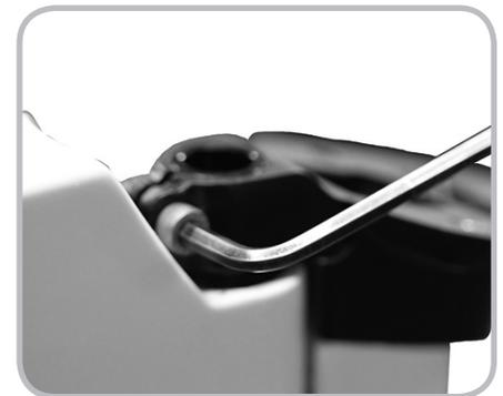
Figure 6.7. Steering axle pinch bolt
