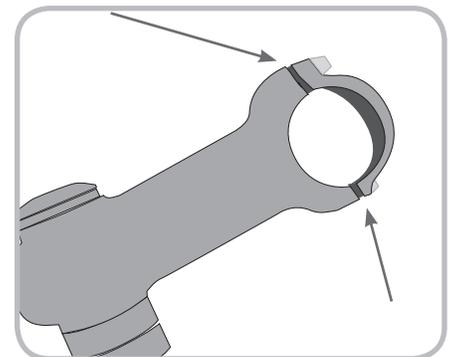
Figure 2.2. Gaps at either end of clamp band
