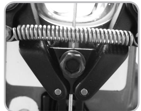
Figure 11.4. Wedge in rollers
