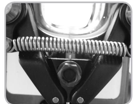
Figure 11.9. Cut cable should not extend past spring.
