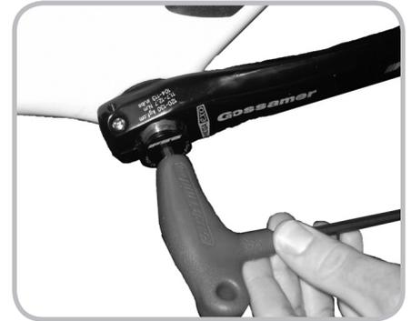
Figure 14.38. Pressing the crank arm onto the axle
