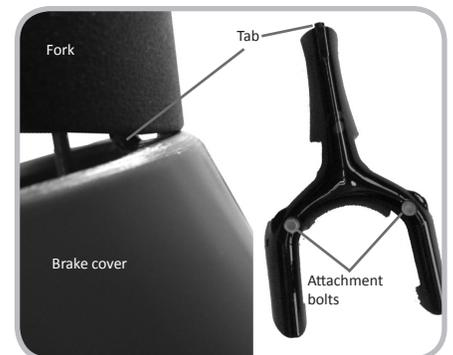
Figure 10.11. Attachment points of front brake cover
