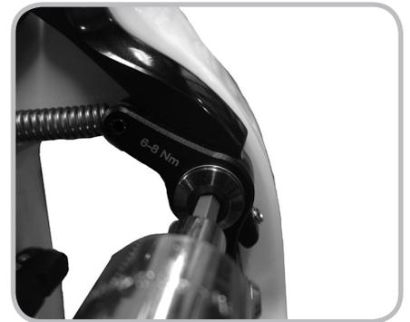
Figure 10.3. Tighten the brake bolts
