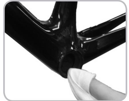
Figure 14.25. Cleaning bonding surfaces with an alcohol wipe
