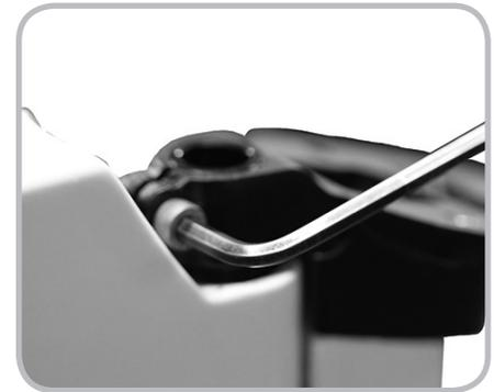
Figure 6.11. Steering axle pinch bolt
