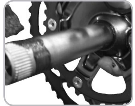
Figure 14.20. Greasing the axle
