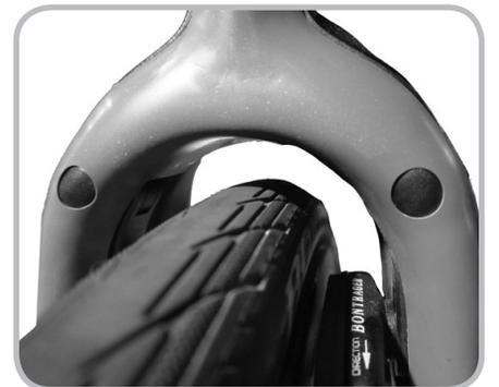
Figure 10.12. Brake cover grommets
