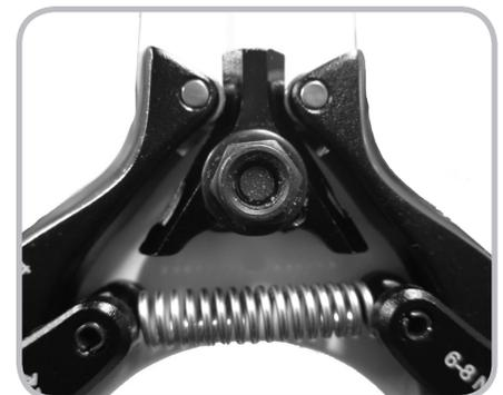
Figure 10.4. Wedge in "home" position between rollers
