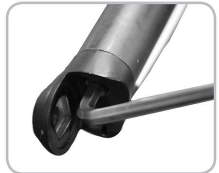
Figure 7.24. Tightening shift lever body
