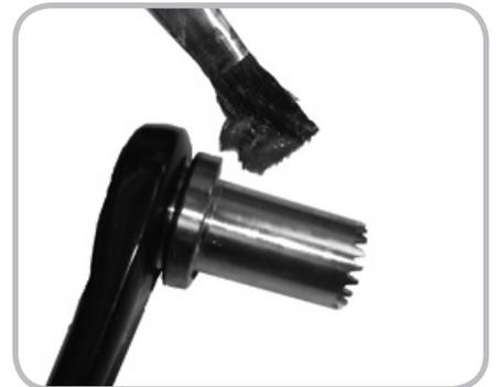
Figure 14.28. Greasing the bearings
