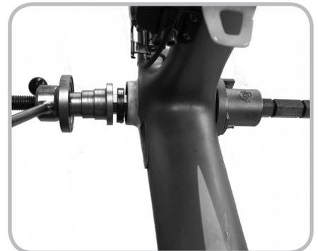
Figure 14.17. Pressing the bearing into the frame
