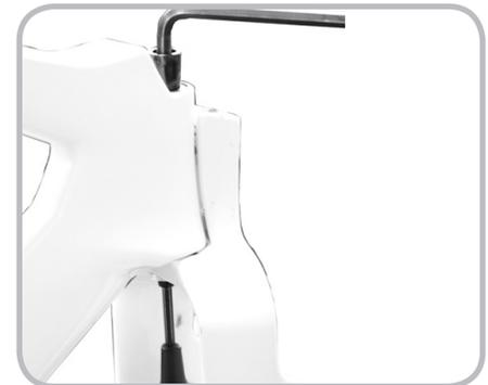
Figure 6.12. Steering axle and steering axle lock bolt
