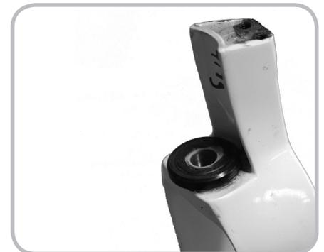
Figure 6.3. Lower head bearing on fork crown
