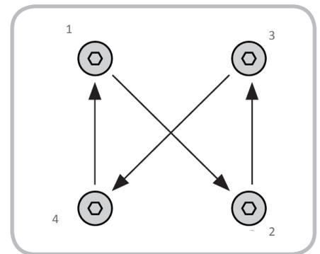
Figure 2.1. Bolt tightening sequence
