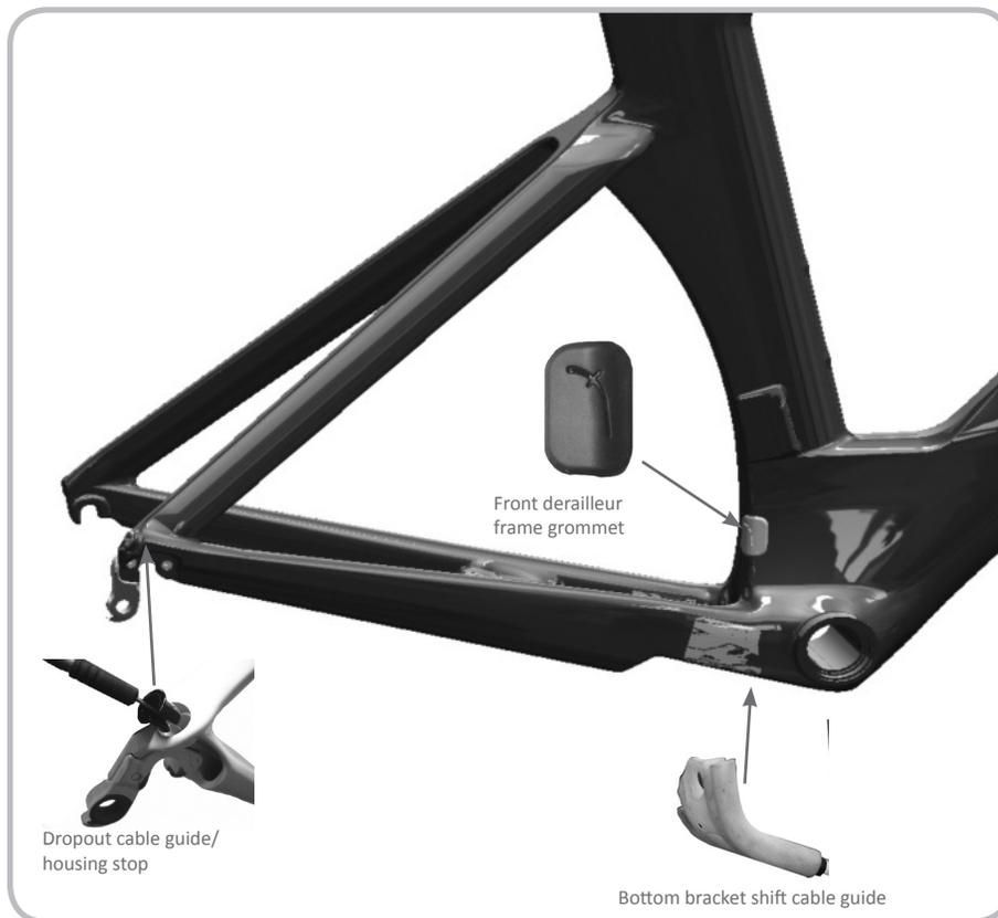
Figure 9.1. Speed Concept parts for shift cable routing
