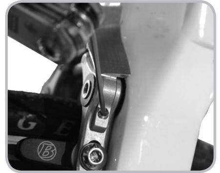
Figure 10.10 Center the brake over the rim
