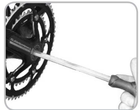
Figure 14.32. Tightening the axle bolt
