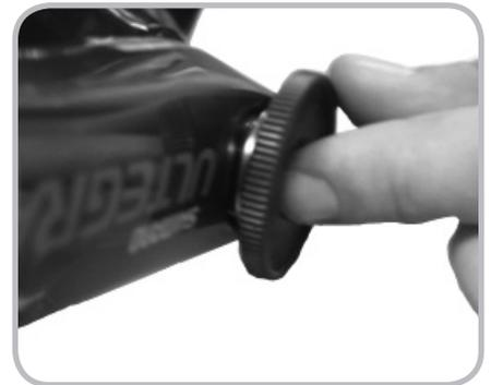
Figure 14.23. Pressing the crank arm onto the axle
