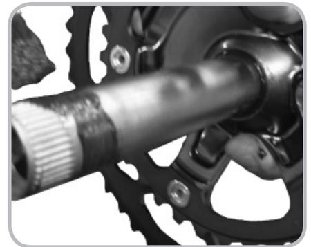
Figure 14.12. Greasing the axle
