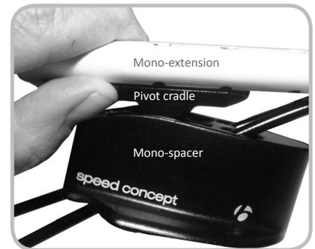
Figure 7.9. Pivot cradle between mono-extension and mono-spacer
