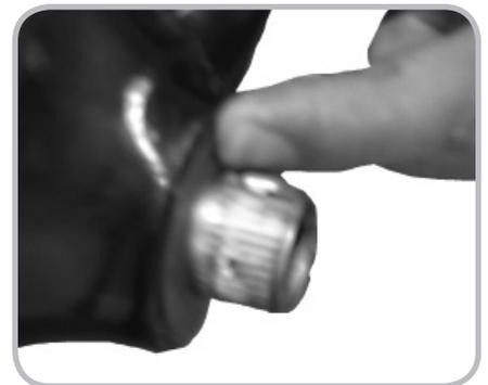
Figure 14.22. Pressing in the second bearing cover
