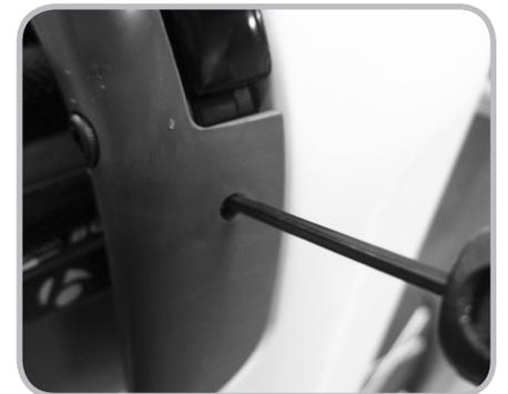
Figure 10.13. Centering screw inside front brake cover
