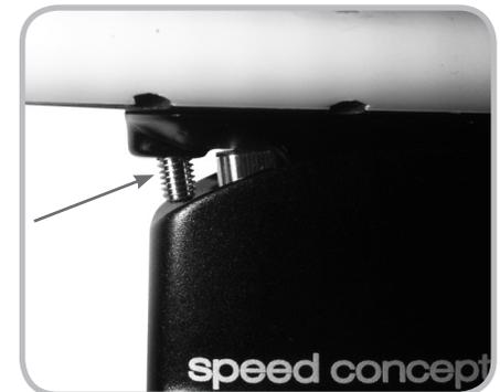
Figure 8.3. Tightening the set screw
