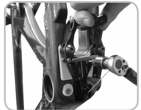
Figure 7.7. Attaching the rear brake
