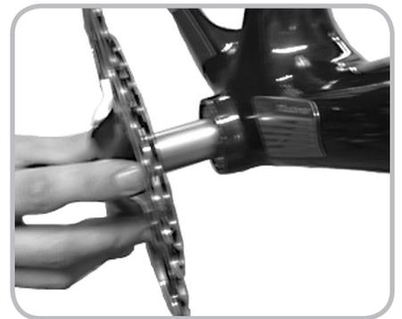
Figure 14.13. Sliding the axle through the bearings
