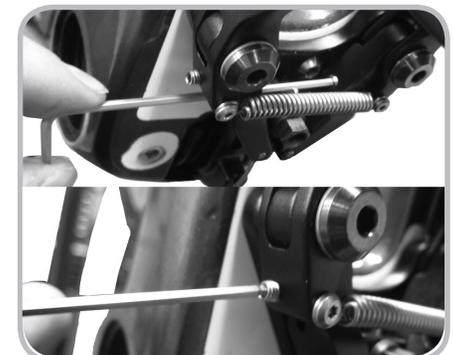
Figure 11.8. Centering the left and right brake pads.
